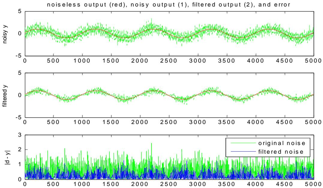
**Figure 27 - LMS equalizer input and the equalized signal.**
