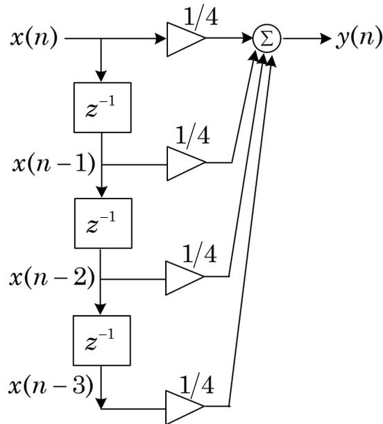
**Figure 11- A Moving Average FIR filter**
