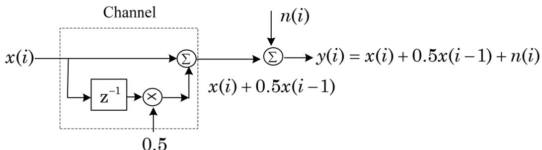
**Figure 16 - A hypothetical channel with additive noise**
