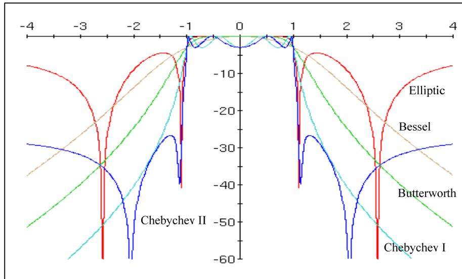
**Figure 10- In-band response comparison**
