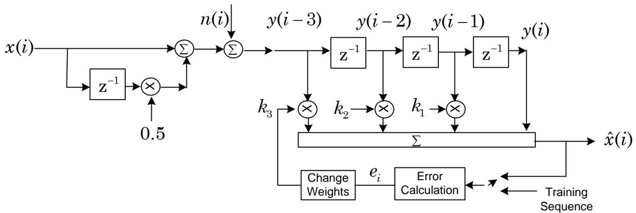
**Figure 19 – A transversal feed-forward adaptive filter**
