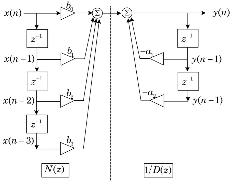
**Figure 13- An IIR filter with both feed-forward and feedback parts.**
