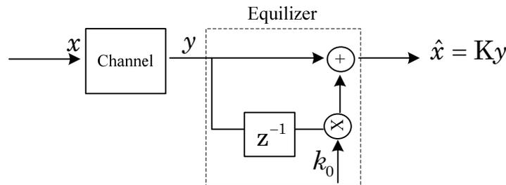
**Figure 17 - The input and output of an equalizer**
