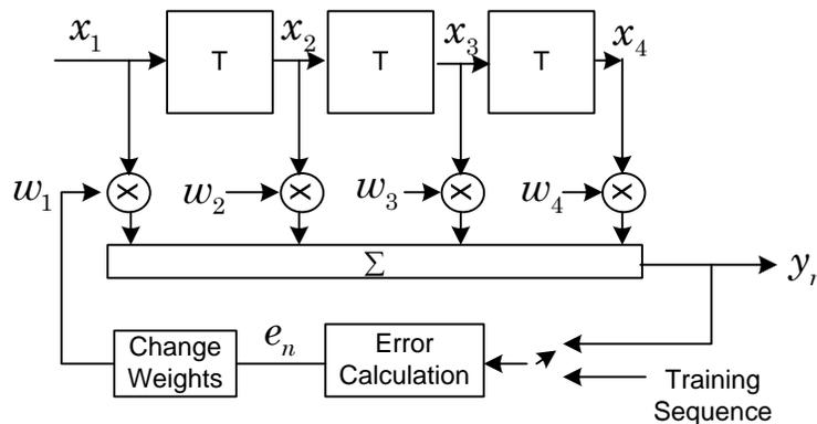
*Figure 21 – Symbol Spaced Equalizer*
