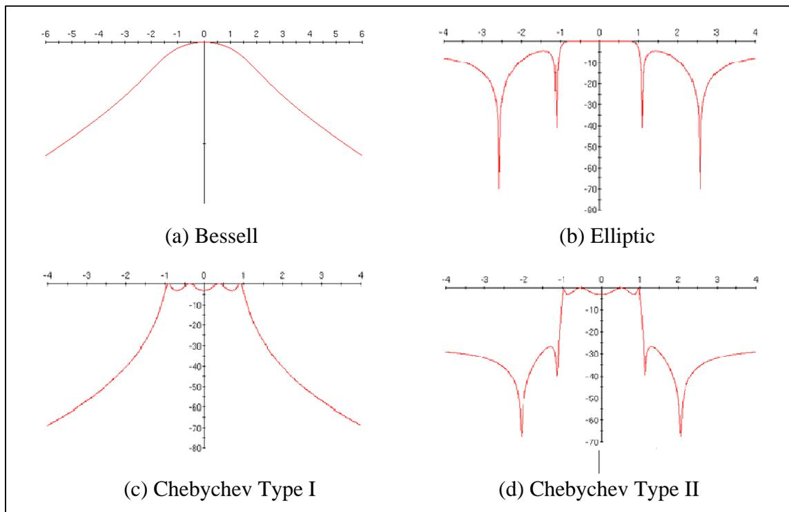
**Figure 9 - The frequency response of (a) Bessell, (b) Elliptic, (c) Chebychev Type I and (d) Chebychev Type II analog filters.**
