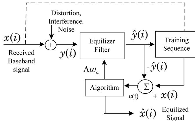
**Figure 15 - Equalization based on a transversal filter**
