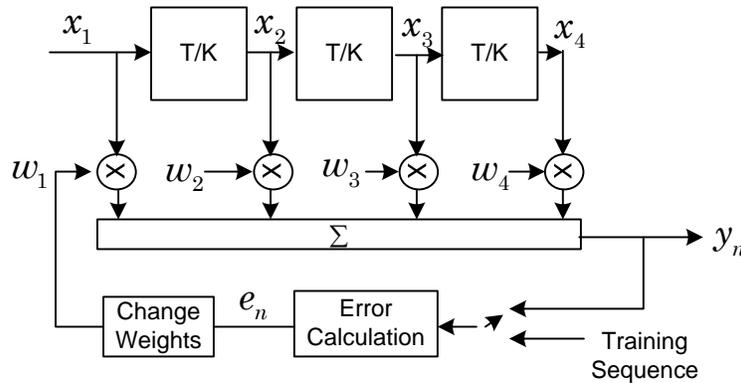
**Figure 22 – A K-fractionally Space Equalizer**
