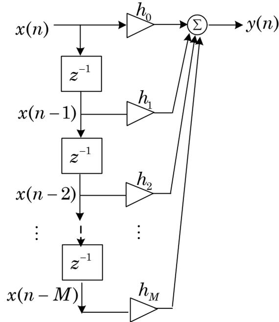
**Figure 12- Generic FIR filter of M+1 taps**
