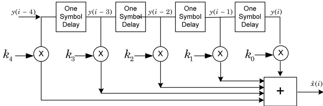
**Figure 18 - Feed-forward filter structure used as an equalizer**
