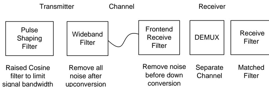
**Figure 1- Uses for filters in a communications chain**
