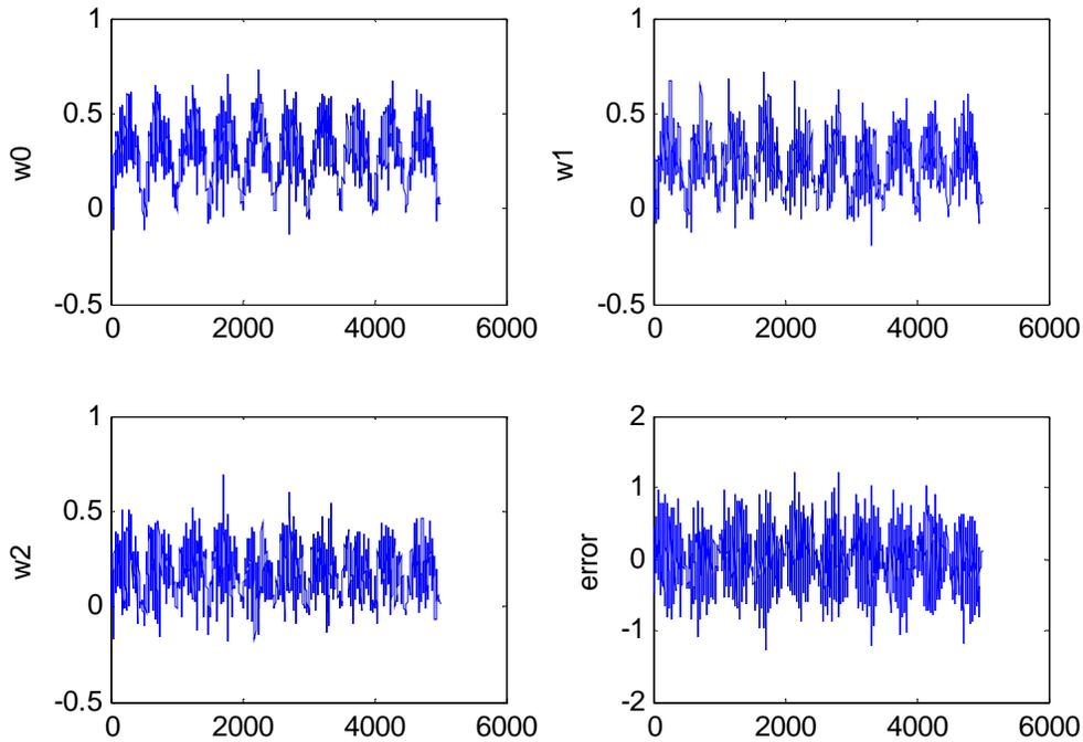
**Figure 28 -The convergence of the filter tap-weights**
