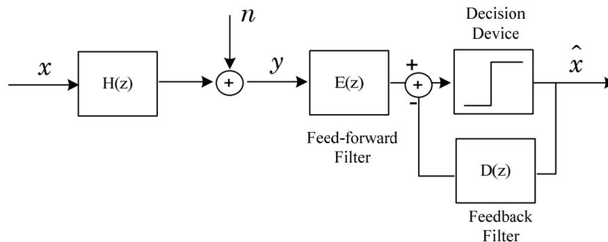
**Figure 23- Dual section DFE Equalizer**
