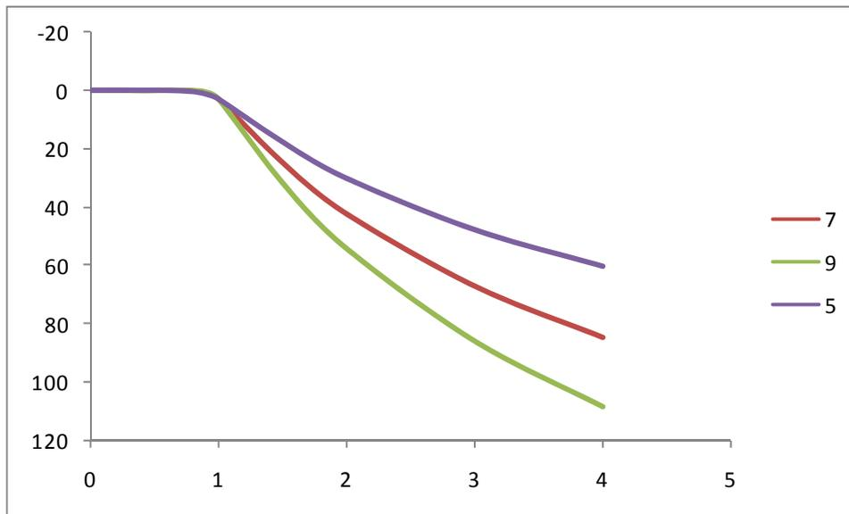
**Figure 7 - Butterworth Filter Frequency Response for order 5, 7 and 9.**
