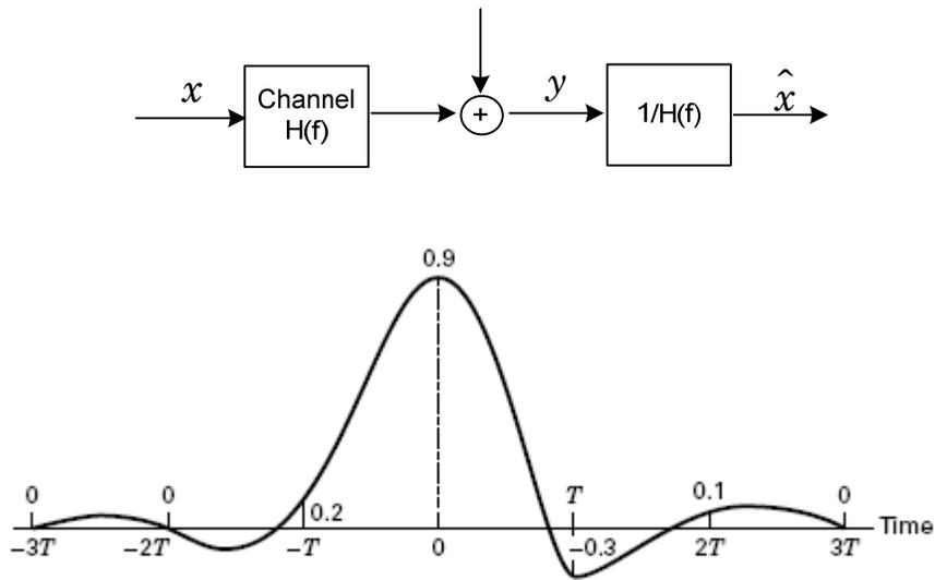
Figure 3.25 Received pulse exhibiting distortion.
