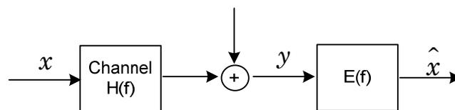
**Figure 14 - Basic idea of an equalizer**
