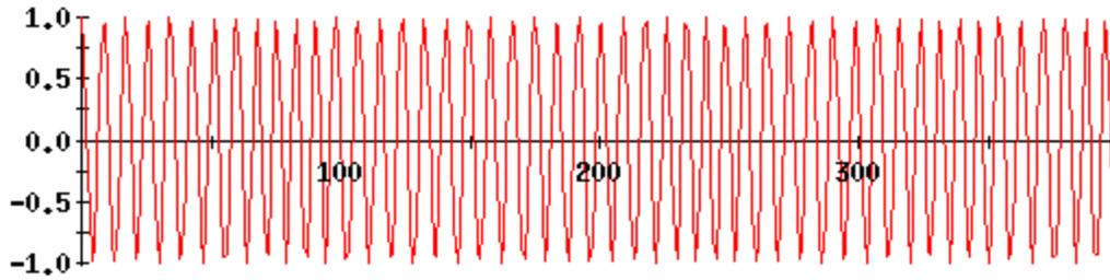
a. MSK modulated signal,  $m(t) = 2.0$ ,  $D\delta f = 1$
