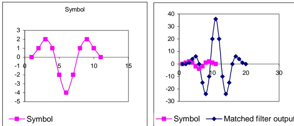
Fig. 13 – A RRC-like symbol and its matched filter output.
