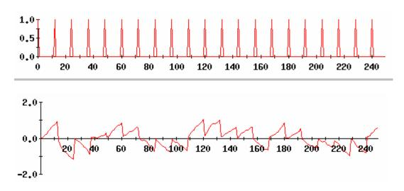
Fig 8 – Integrate and Dump output
