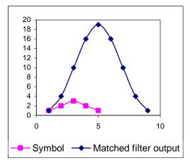
Fig. 9 – A triangular pulse and its matched filter output
