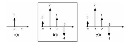
Fig. 3 – The LTI transforms an incoming signal based on a fixed rule.
