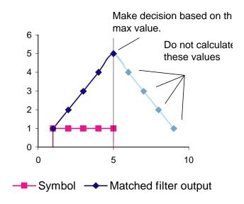
Fig. 6 – A square pulse and its matched filter output.
