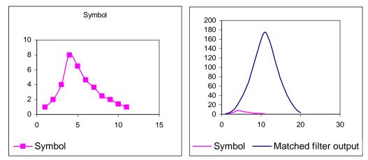
Fig. 15 – An unsymmetrical received signal and its matched filter output.
