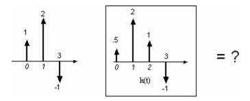
Fig. 4 – Putting a signal composed of many pulses through a LTI
