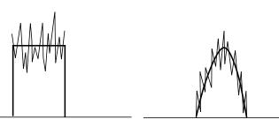
Fig. 10 – The effect of noise on the average signal to noise ratio is different for these two pulses.
