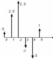
Fig 5d – All responses added up to give the combined response to three pulses.
