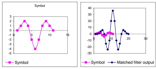
Fig. 13 – A RRC-like symbol and its matched filter output.
